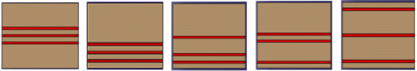
Fig. 4. Several samples of FRP layer with three glass fiber layers.
