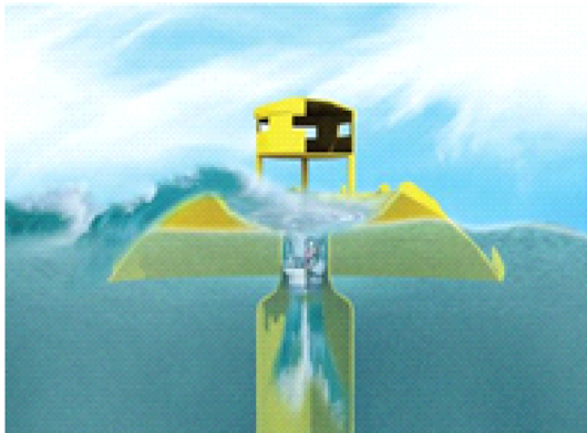
Fig. 1. Spiral-reef overtopping device (single-stage OWEC type) (Nam et al. [2008]).
