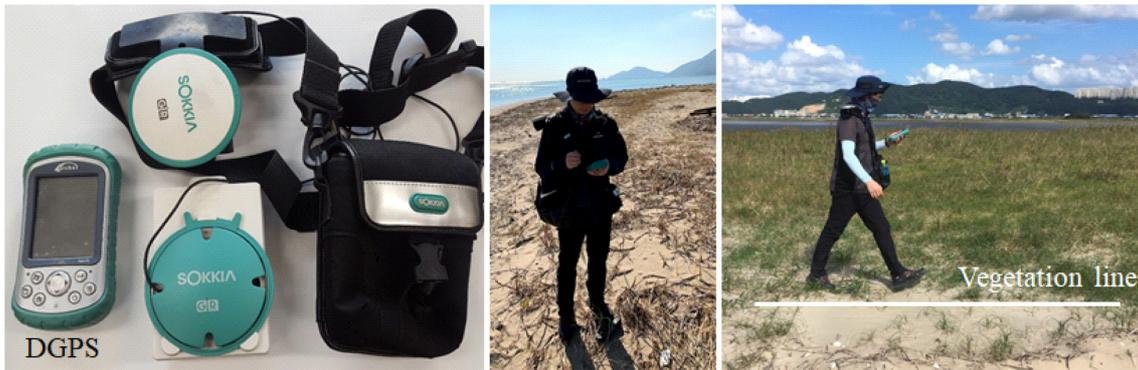
Fig. 2. Composition of DGPS used for fieldwork and trace of vegetation line.
