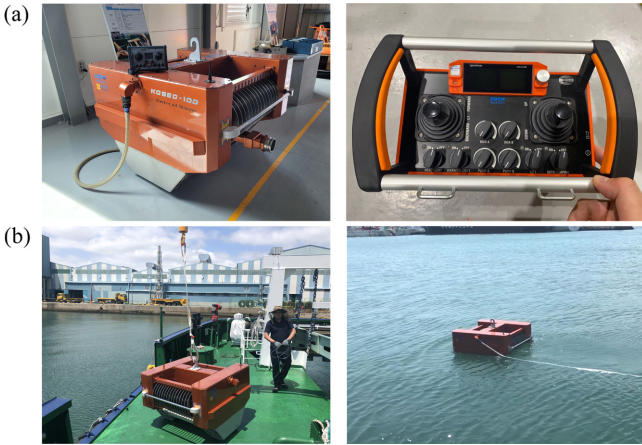
Fig. 2. The photograph of (a) the final production of rotary disk oil skimmer (KOSED-100) and (b) the scenes of KOSED-100 being tested in the field.
