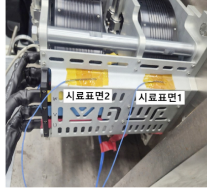
Fig. 7. Locations of temperature measurement points (specimen surface 1 and 2).
