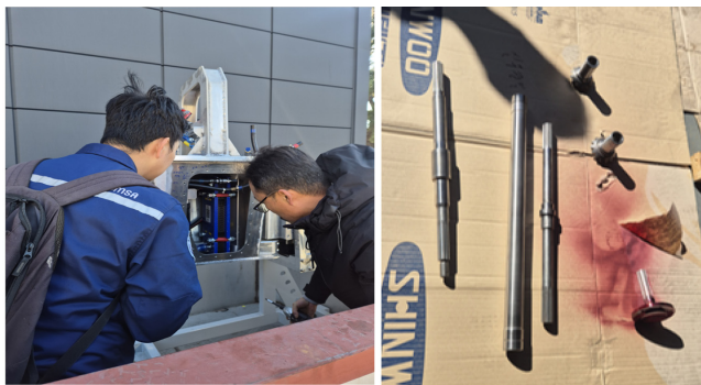
Fig. 8. Visual and PT Inspection.
